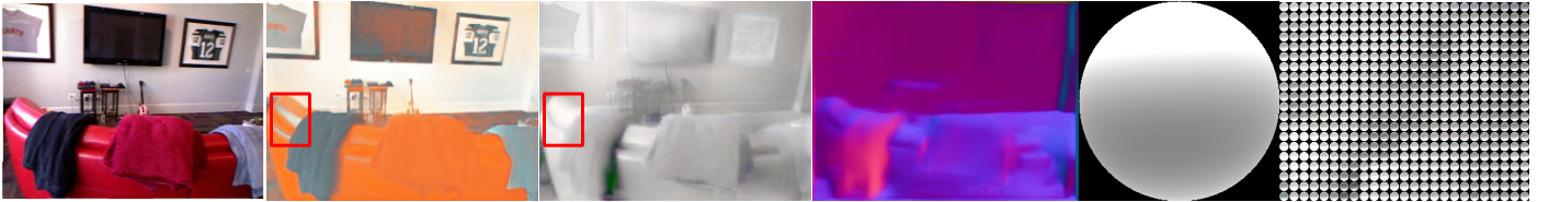
Figure 10. From left to right: input image, reflectance, shading, normal, global SH and local SH predicted by the proposed method. Note that the specular effect appears in the predicted reflectance.
